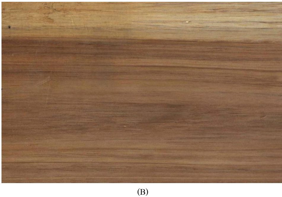
Figure 1. Cross section lumber and see heart rot at central log (A) and flat sawn board, tangential section (B) of Acacia mangium Willd.
